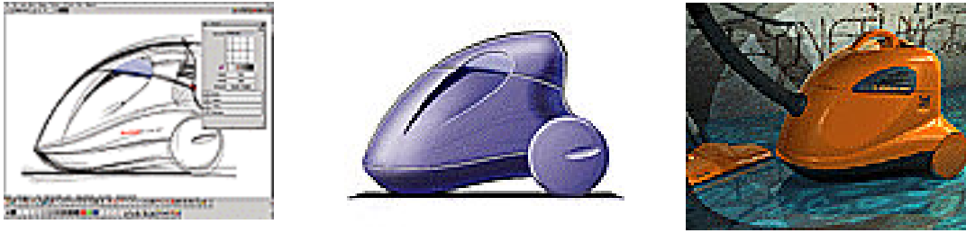
Fig. 7. (a) Sketch the product, (b) Colour and texture mapping, (c) Rendering of the 3D Model.
